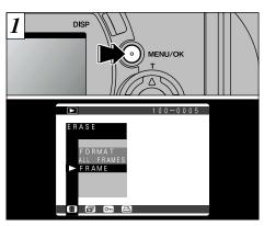
Press the "MENU/OK" button to display the menu on the monitor.
